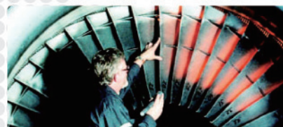
Turbine blades after repair treatment
